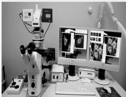
An experimental chamber (500  $\mu$ l) with a suspension of cells was placed on the slide of an inverted microscope Axiovert 100M with a laser scanner LSM 5 (Zeiss, Oberkochen, Germany). Confocal images were obtained with a Zeissplan-Apochromat 40x1.4 lens. Visualization of changes [Ca<sup>2+</sup>]<sub>i</sub> was performed using high-affinity (kd = 325 nM) Ca<sup>2+</sup>-sensitive fluorescent dye a Fluo-3 AM (максимуми абсорбції/емісії=506 нм/526 нм).
